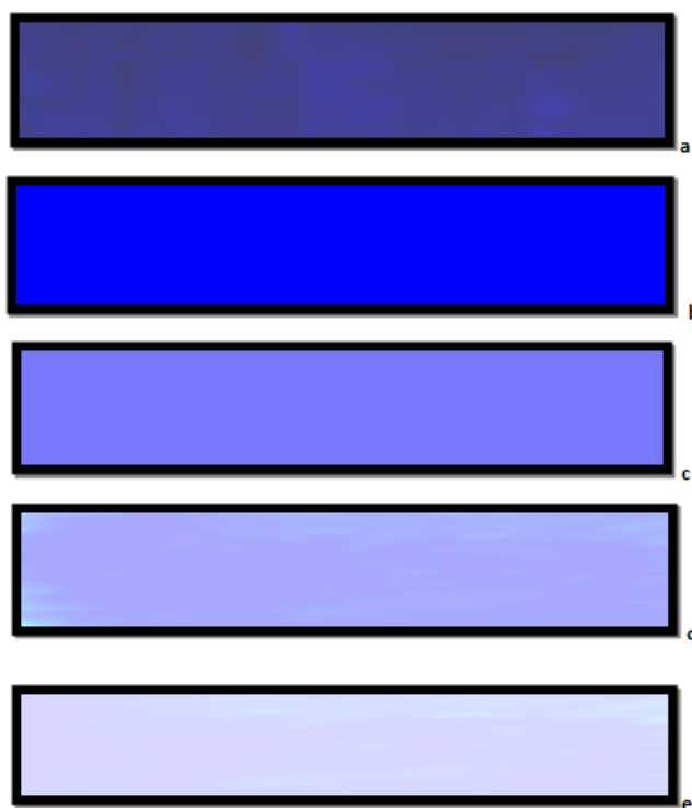
Fig. 9: The coated metallic surfaces with different colored pigments. a- CoAl_2O_4 + Co_3O_4 , b- CoAl_2O_4 , c- Co_{0.75} Mg_{0.25} Al_2 O_4 , d- Co_{0.5} Mg_{0.5} Al_2 O_4 , e- Co_{0.25} Mg_{0.75} Al_2 O_4
