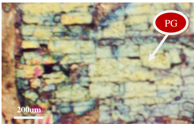
Fig. 12a: Microphotograph of thin section of the internal part of NPK fertilizer showing the table's structure of PG filler.
