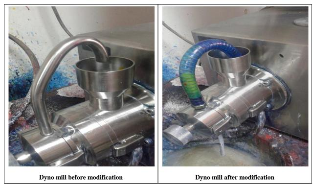
Fig. 2: Dyno mill (mini motor mill) before and after modification by flexible hose.
